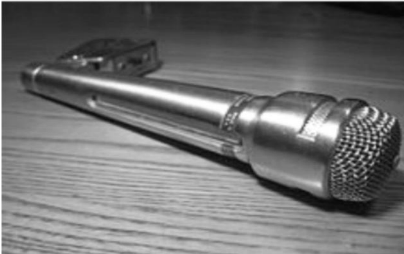
Fig: A commonly used dynamic cardioid microphone.
