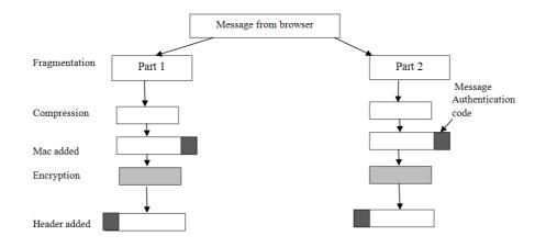
Figure 9. 3: Data transmission using SSL
