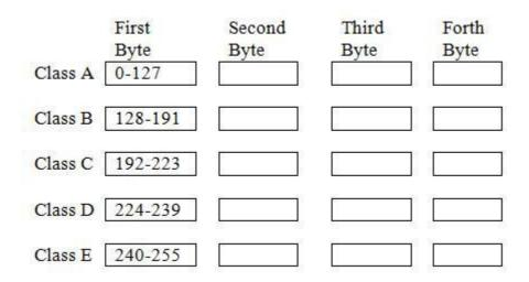
Fig.3.3 Determining the classes using dotted-decimal
