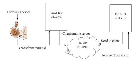
Figure 1.5: Establishing TELNET Connection
