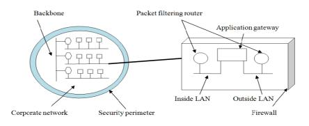
Figure 9. 4: A firewall consisting of two packet filters and an application gateway
