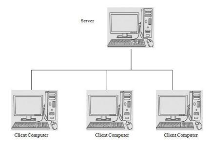
Figure 1.2: Connecting nodes in Client Server Mechanism
