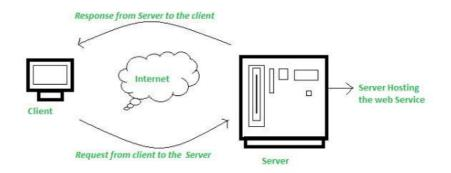
Fig.2.2 The Operational Process of a Web Service.
