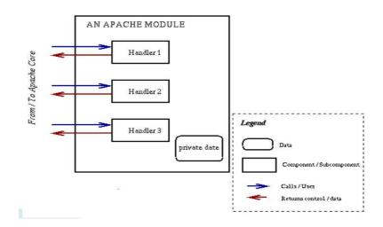
Fig.3.5 Handler system within an Apache Module
