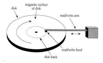
Figure 1.6: A Typical Disk Drive
