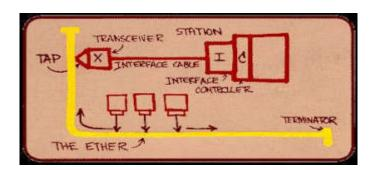
**Figure 3.** A 1976 drawing by R. Metcalfe of the Ethernet concept (from Charles Spurgeon's Ethernet Web Site)
