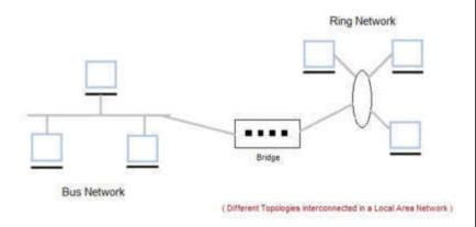
Fig. 2.1 Block Diagram of LAN
