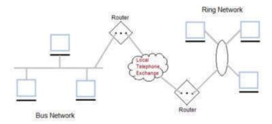
Fig. 2.2 Block Diagram of MAN
