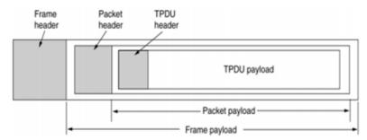
Figure 4.1: The nesting of TPDU, Packet and Frame
