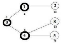
Next, select the vertex with minimum distance value which is not already included in the SPT. The vertex 5 is selected and inserted into SPT. Now the SPT becomes [0, 1, 4, 5]. The distance values of the adjacent vertices of node 5 are updated. So, the distance value of node 6 is updated as 11 and the distance value of node 8 is remained unaffected.
