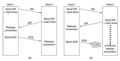
Figure 4.8: (a) Normal case of Three-way handshake (b) Final ACK lost
