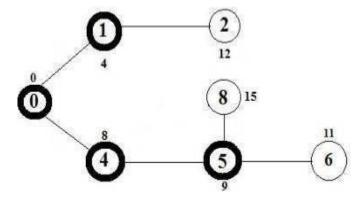
The steps are repeated iteratively until we get all the vertices inserted in the SPT. Finally, the following SPT is found:
