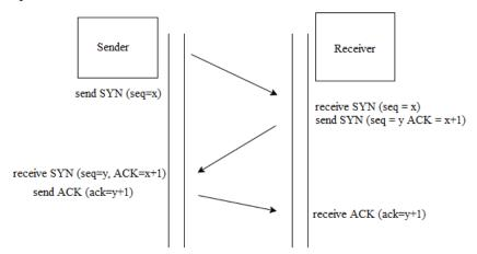
Figure 5.4: TCP 3-way handshaking
