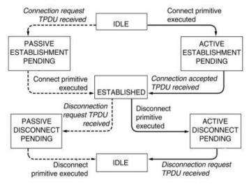
Figure 4.2: State Diagram of Simple Connection Management Scheme
