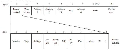
Figure 5.8: The data frame structure of 802.11
