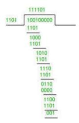
From the above calculation, we have seen that the remainder is 001. Therefore, the encoded data sent is 100100001.
