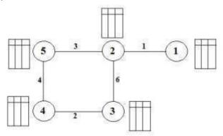
The above network has 5 routers and each router has its own routing table. A routing table as shown below contains at least three entries.
