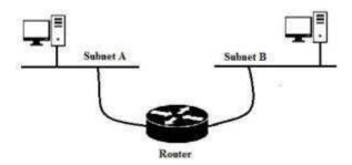
Fig 2.2: Different subnets connected by Router
