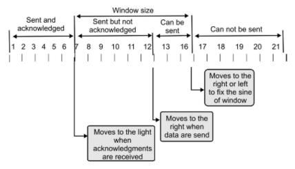
Figure 4.12: Sliding Window for Flow Control
