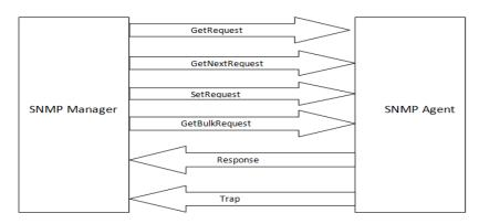
Figure 7.4: SNMP different data packets or PDUs
