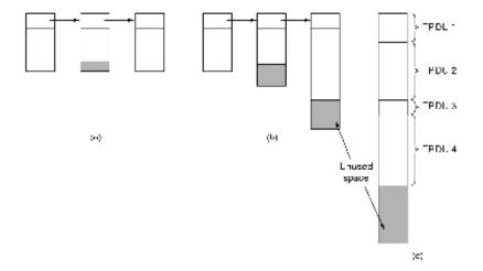
Figure 4.13: (a) Chained fixed-size buffers. (b) Chained variable-sized buffers. (c) One large circular buffer per connection.
