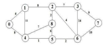
For the above weighted graph let's consider the Node 0 be the source node from which the shortest paths to all other vertices are to be found using Dijkstra's algorithm.
