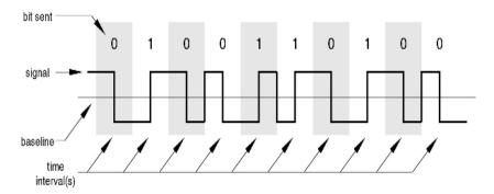
Figure 4.5: Encoding of Signal in Manchester Encoding
