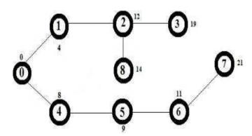
The weights written outside the nodes indicate the shortest distance from the source node (node 0) in the above example.
