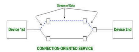
Fig. 2.4 Block Diagram of Connection-oriented Networks
