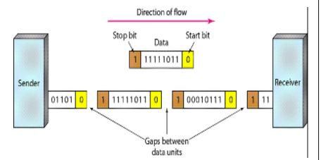
Fig 6.5: Asynchronous transmission (Source: Internet)
