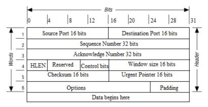
Figure 5.3 Structure of TCP segment
