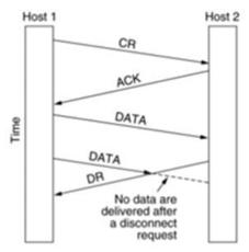
Figure 4.7: Disconnection with loss of data
