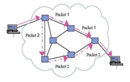
Figure 2. Packet switching Network
