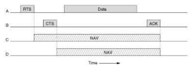
Figure 5.4: The virtual channel sensing using CSMA/CA
