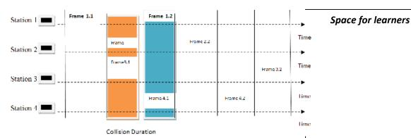
Figure 3.4 Frame collisions in slotted ALOHA
