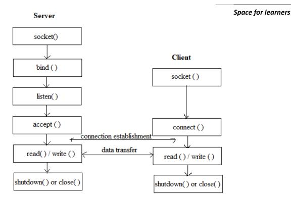
Figure 5.6 Communication using socket
